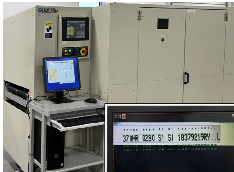
Laser etched barcoder for material traceability.
