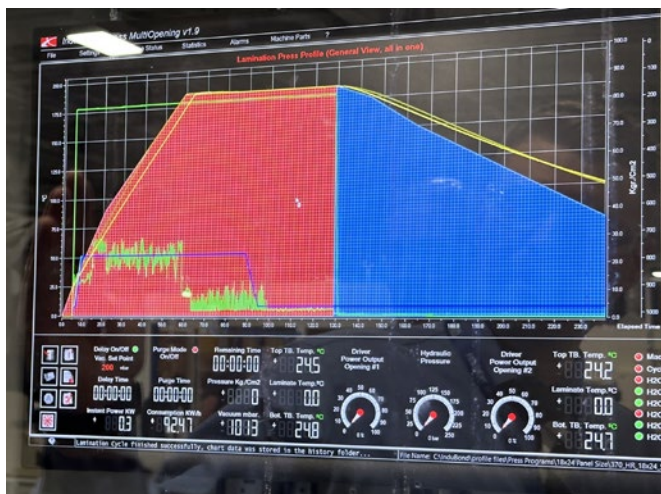
InduBond lamination press profile data.
