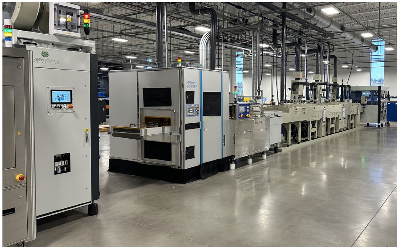
Right to left: GSE double loader, followed by Chemcut preclean line, electrostatic cleaner and preheat oven, cut-sheet laminator, GSE UV-protected lift-up gate, GSE FIFO FILO-capable buffer with cooling, and partial view of Mylar peeler.
